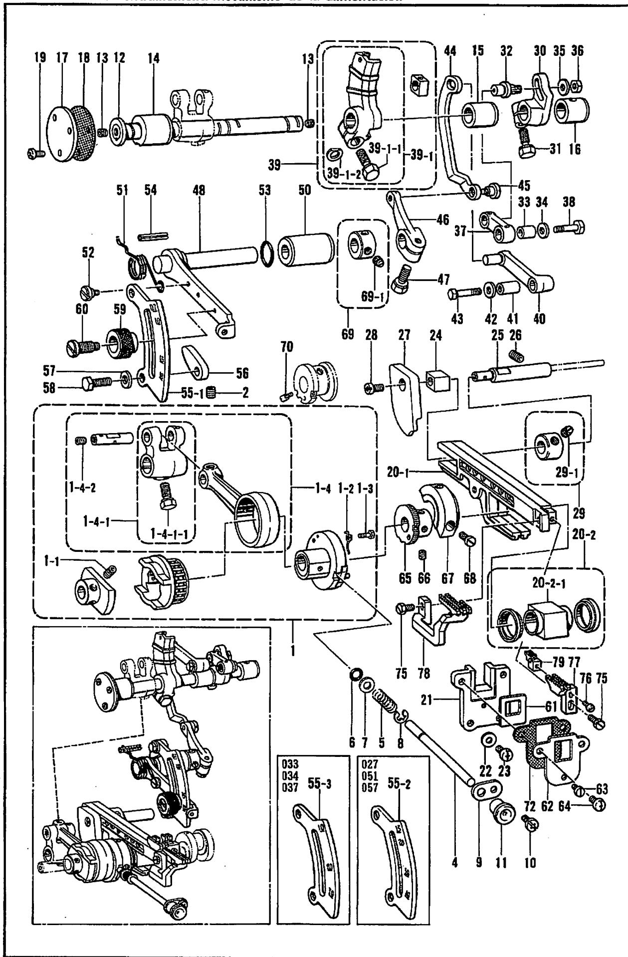
F. 送り関係/Feed mechanism/Transportvorrichtung/
