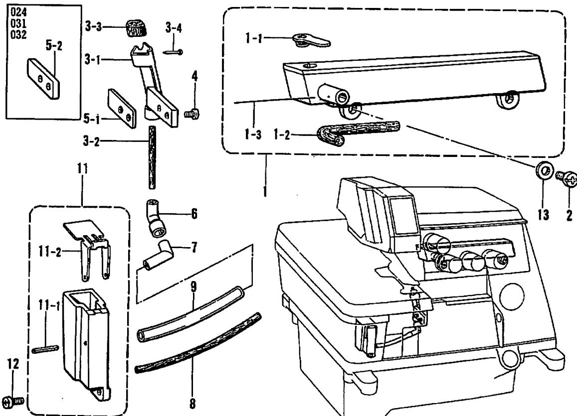
B. 駆動軸関係/Crank shaft mechanism/Kurbelwelle/
