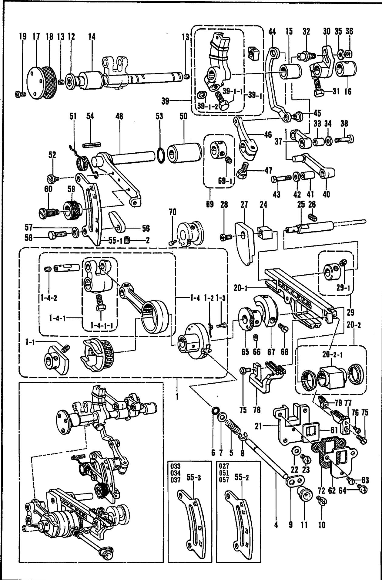
F. 送り関係/Feed mechanism/Transportvorrichtung/
